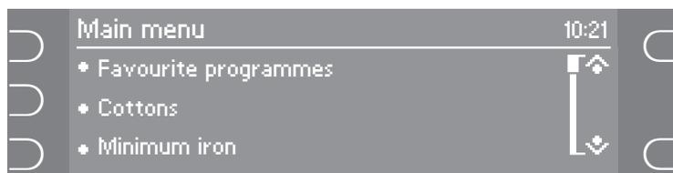
The sensors on the right can be used to scroll up or down the list. Each touch of the sensor will move the list up or down one line.
