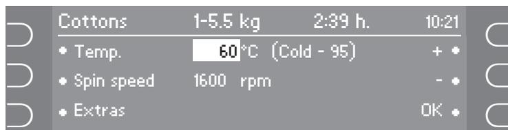
Use the sensors on the right to increase (+) or decrease (-) the value highlighted (60). The altered value must then be confirmed with the lower right sensor **OK**.
