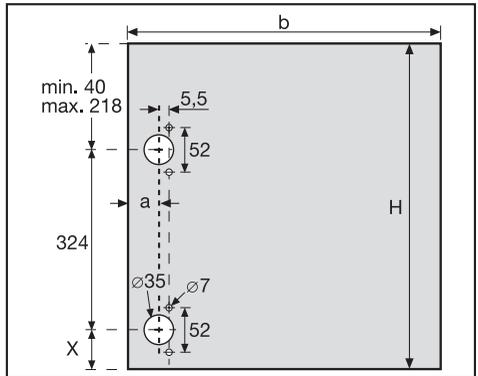
if width (**b**) increases, measurement **a** must also be increased
