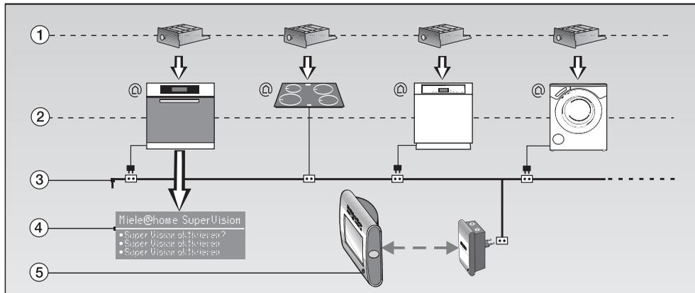
This washing machine is communication enabled and can be linked into the Miele@home system via a communication module ① (optional accessory).
