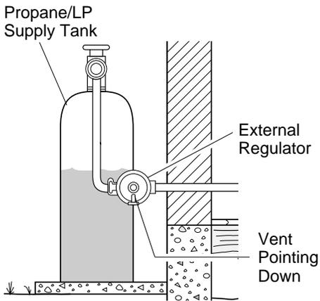
**Figure 20 - External Regulator with Vent Pointing Down**
