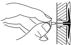
Figure 15 - Popping Open Anchor Wings For Thin Walls
