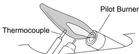
Figure 26 - Correct Pilot Flame Pattern
