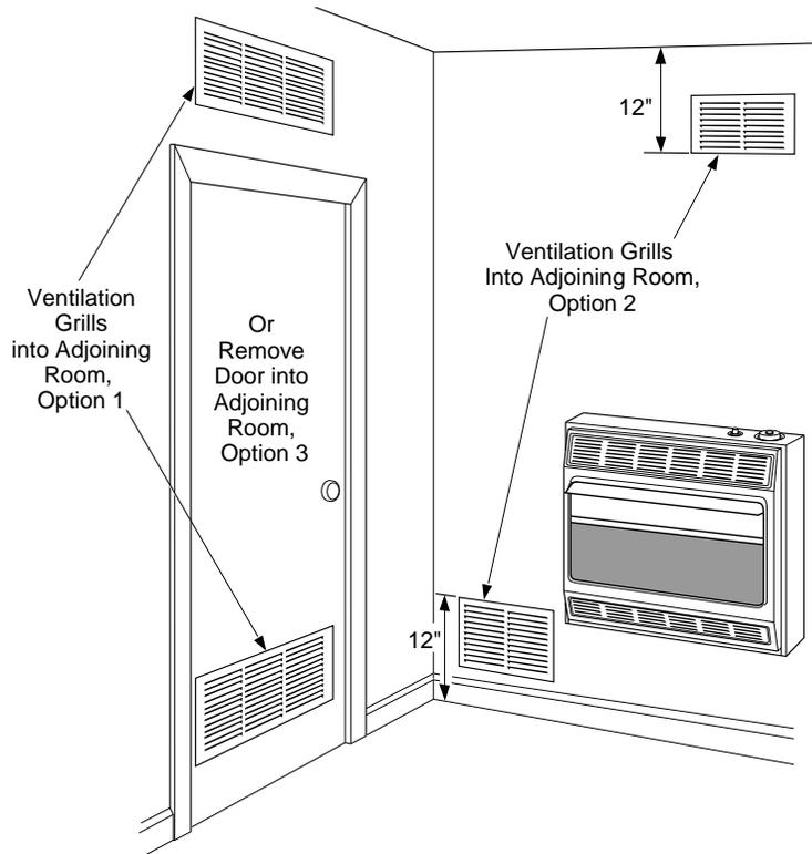
Figure 8 - Ventilation Air from Inside Building
