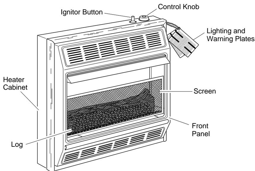
Figure 1 - Vent-Free Gas Log Propane/LP Gas Space Heater
