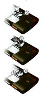
Open the cover and insert the memory card with the gold-coloured contacts facing down.
