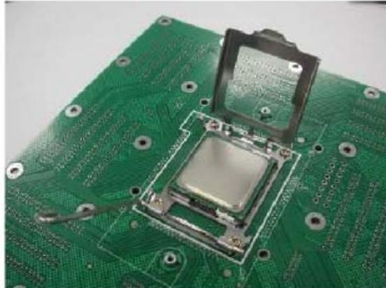
7. Close the socket. Rotate the load plate onto the package lid. Engage the load lever while pressing down lightly onto the load plate. Secure the lever near the hook end under the retention tab.
