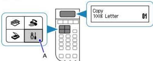
1. Press the **Setup** button (A) on the printer.
