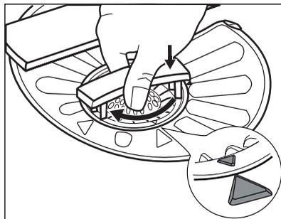
1. Turn the filter (A) counter-clockwise and remove it.
