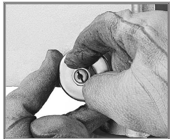
Figure 32. Loosening spring nut.
