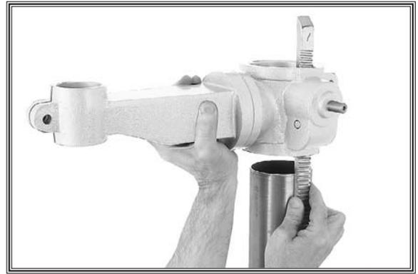
**Figure 11.** Sliding table bracket and rack over column.
