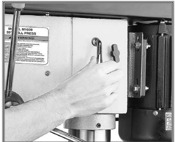
**Figure 24.** Using the belt tension lever.
