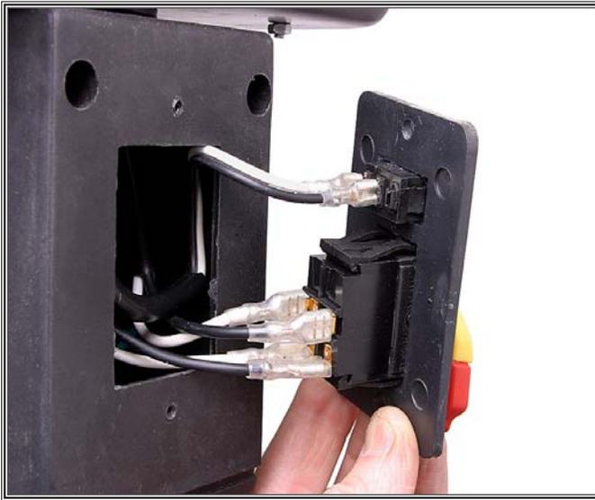
Figure 33. Power and light switch wiring.
