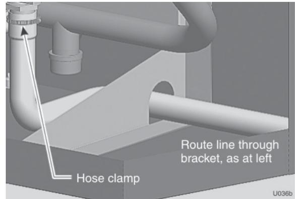
**Figure 13** Condensate drain — Ultra-155 & -230 (PVC tee installation shown applies to all models))
