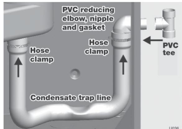
**Figure 14** Condensate drain — Ultra-310
