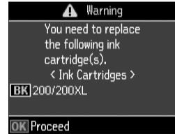
If you're replacing a cartridge before you see a message on the LCD screen, press **⏠** if necessary and select **⚙ Setup**. Select **Maintenance**, then select **Ink Cartridge Replacement** and press **OK**.
