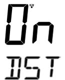
A digital display showing 'ON' in the top row and 'DST' in the bottom row, indicating that Daylight Saving Time is currently set to 'ON'.
