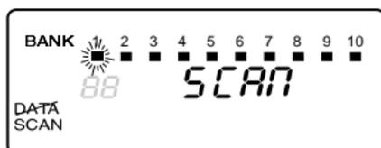
2. The bank indicators selected for scanning appear in the display, and the bank being currently monitored flashes. You can deselect banks from active scanning by pressing their number on your keypad. The indicator for each deselected bank turns off, and the bank's channels are not scanned.
