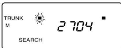
*The ID is locked out, and the next active ID displays. You can lockout up to 200 IDs.*
