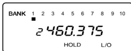
3. Press **(L/O)** to unlock the channel. The **L/O** icon goes out.
