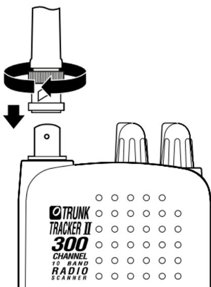
Attach the flexible antenna to the BNC connector.
