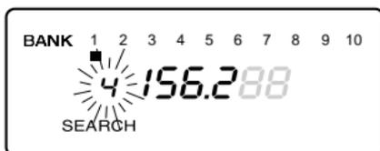
When data skip is active, your scanner may pause momentarily on an unwanted signal but will resume searching in 2 or 3 seconds. Data Skip does not function when the **AIR** Band is selected.
