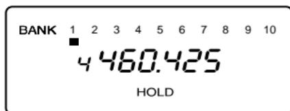
3. Press and hold **(PRI)** / **TURBO** for two seconds to designate this channel as your new Priority Channel.
