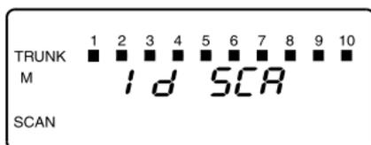
2. To remove a Scan List from active scanning, press the number of the Scan List on your keypad.
