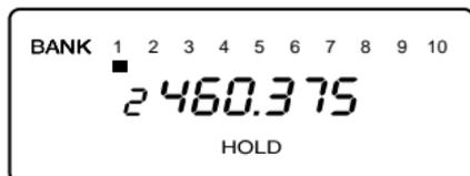
3. Press **(L/O)** to lockout the channel. L/O appears in display.
