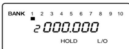
**Note:** *Channels with no frequencies are automatically locked out.*
