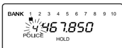
2. Locate the lock-out frequency using ▲/▼.
