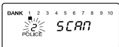
3. Press (SVC) to scan the RR band. When an active channel is displayed, the scanner will alternate between the frequency and the Railroad channel number.
