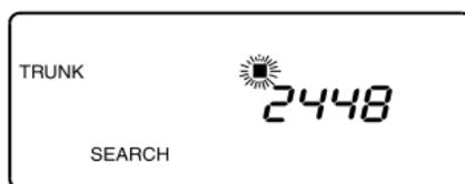
**Note:** *If you lockout an ID in Search mode, it is also locked out in Scan List mode. Conversely, if you lockout an ID while in Scan List mode, it is locked out in Search mode. For information about Scan Lists see page 48.*
