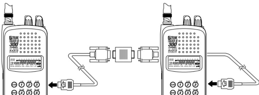
Plug the smaller end of each of the supplied Remote interface cables into the remote ports which are on the right sides of each of the two scanners.
