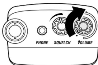
3. Think of the Squelch Control as a gate. Turn **SQUELCH** fully counter-clockwise. This raises the "Squelch Gate" so high that only very strong signals can get through.
