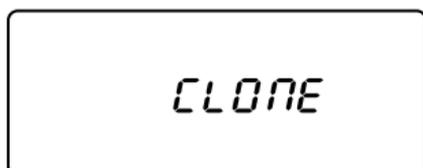
5. Press the **(DATA)** key on both scanners. The data transfer is started from the "First" unit to the "Clone" unit.
