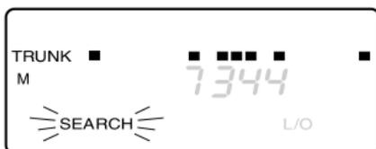
**Note:** Locked out IDs display during ID Monitor mode with the **L/O** icon turned on.
