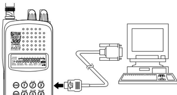
Plug the smaller end of the supplied Remote Interface cable into the remote port which is on the right side of the scanner. Plug the other end of the cable (DB-9 serial connector) into a personal computer's serial port. A few PC's may require an adapter, most will not. Of course, make sure your PC is turned on.
