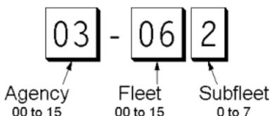
Assuming that you have the system frequencies programmed, and your scanner is locked to the control channel, you can select a desired city by simply searching on the AGENCY part of the AFS talk group number. For example, you can select the entire city of Sullivan with 4 key presses - zero, three, dot, SRCH.
