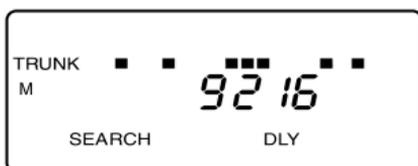
**Note:** *If more than 20 channels are stored in a bank, then the indicators represent multiple channels. For example, if 28 channels are programmed, the first 8 activity indicators each represent two channels.*
