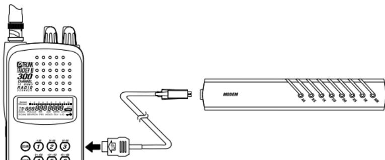
Plug the smaller end of the supplied Remote interface cable into the remote port which is on the right side of the scanner. Plug the other end of the cable (DB-9 serial connector) into the external modem. You may need a DB-9 to DB-25 null modem adapter, available at most computer stores. Of course, make sure your external modem is turned on. Make sure that you have a phone line plugged into the modem jack on the back.
