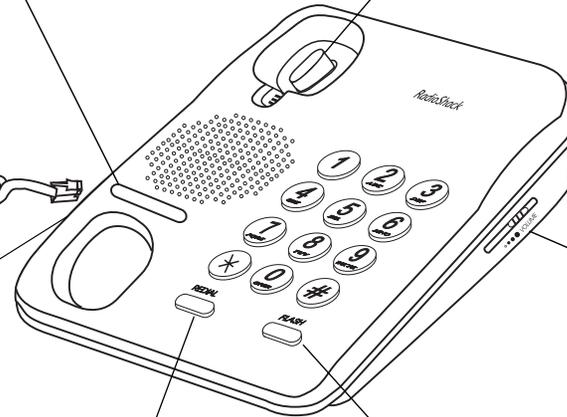
Plug the handset cord into the jacks on the base and handset.
