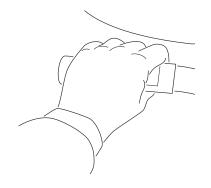
**NOTE:** The Contact Hand Pulse Sensors will work for the HRT® programs, but it is recommended to use the telemetric chest strap for an uninterrupted signal and ease of use.
