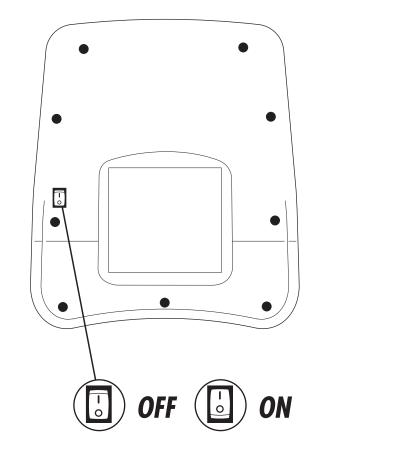
**ON/OFF SWITCH** Turn your Incline Elliptical Trainer off if you will not use it for an extended period of time.
