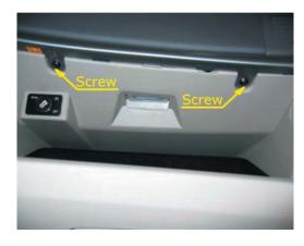
Remove 2 screws and use plastic wedge to remove plastic rim.
