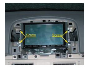
Tighten headunit with 4 screws.
