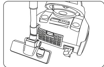
**NOTE:** When rewinding the power cord, guide the cord with one hand. This will prevent the cord from whipping which could cause damage or injury.
