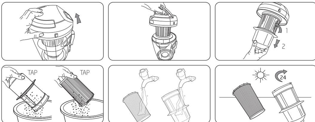
**Cleaning the Post-Motor Filter****NOTE :** This is located at the rear of the vacuum cleaner.
