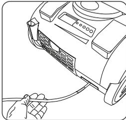
**NOTE:** Fully unwind the power cord. A yellow mark on the power cord indicates the recommended cord length. Do not exceed the cord length beyond the red mark.
