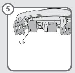
Install a light bulb in each socket.
