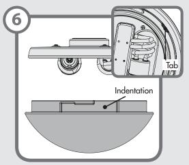
Installing the globe- Position the indentations in the outer rim of the globe so that they line up with the tabs on the inside surface of the light fixture rim. Carefully lift the globe up inside the light fixture as far as it will go. Rotate the globe in a clockwise direction until it is held tightly in place by the four tabs.
