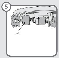
Install a light bulb in each socket.
