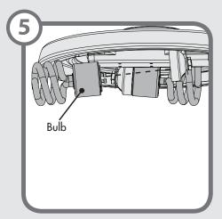
Install a light bulb in each socket.
