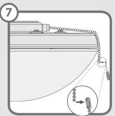
Installing the pull chain pendant Attach the pull chain pendant to the
