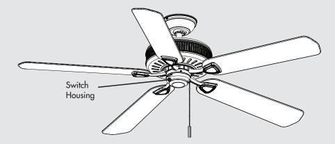
Your light kit is compatible with most ceiling fans. The light kit will attach to the fan's switch housing. Begin on page 3 where you will choose the type of switch housing that most closely resembles the one on your fan. From there, you will be directed to the set of assembly instructions that are appropriate for installing the light kit to your fan.
