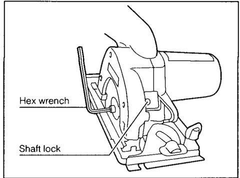
To install the blade, follow the removal procedure in reverse
