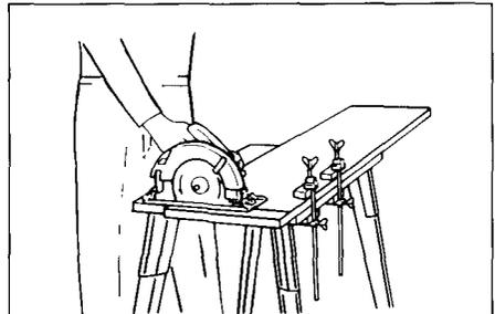
A typical illustration of proper hand support, workpiece support, and supply cord routing.
