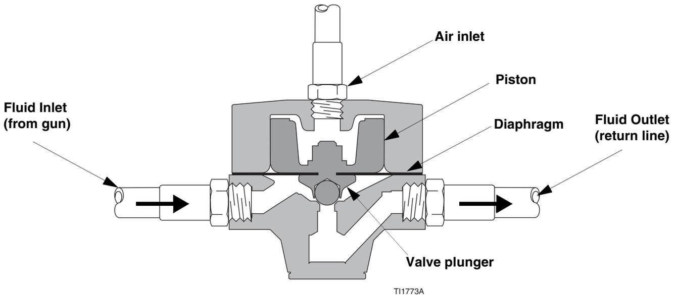
Fig. 1. Cutaway of Pneumatic Back Pressure Regulator
