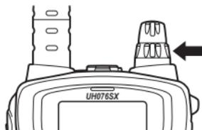
To set the "Squelch Gate" to the desired level, turn **[SQ]** counter-clockwise until you hear noise. Then turn the **[SQ]** clockwise just until the noise stopped. Now only the desired signal can get through.
