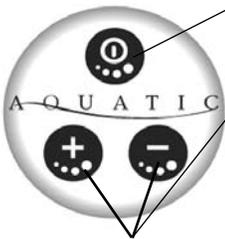
**On/Off Button:** The blower can be turned on or off by pressing this button. Press the button once and the blower will turn on. Press the button again and the blower will turn off.
