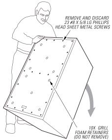
To do this the enclosure will first be rested on its back, the grille removed, and the HF horn assembly disconnected, removed, and disassembled. Its rear bracket will be re-installed into the new KF850z HF horn assembly, which will then be installed into the enclosure.
