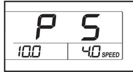
Each program consists of 30 one-minute periods. One speed setting is programmed for each period. Note: The same speed setting may be programmed for two or more consecutive periods. The profiles on the console show how the speed of the walking belt will change during the programs.
