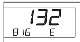
**IMPORTANT:** If a “d” appears in the lower right display, the console is in the “demo” mode. This mode is intended to be used only when a treadmill is displayed in a store. When the console is in the demo mode, the power cord can be plugged in, the key can be removed from the console, and the display will remain lit, although the buttons will not operate. **If a “d” appears when the information mode is selected, press the Speed decrease button so the “d” disappears.**
