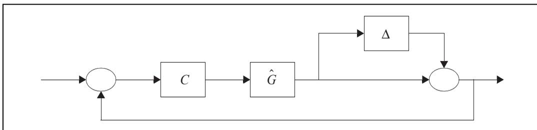
**Figure 3-1.** Controller  $C(s)$  Designed for Multiplicative Error Reduction
