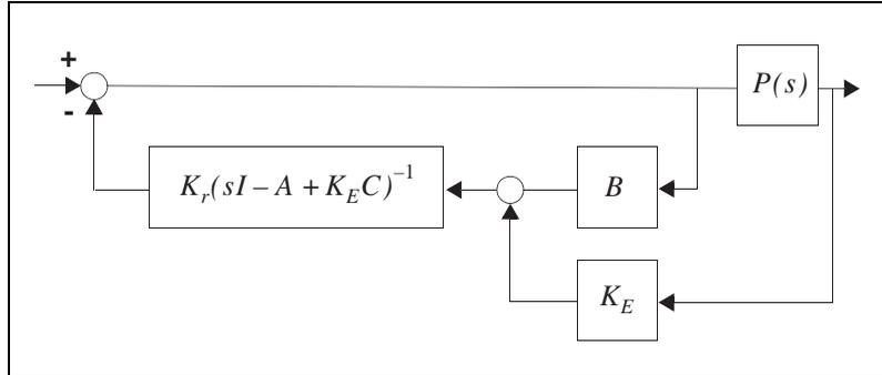
**Figure 4-3.** C(s) Implemented to Display Left MFD Representation
