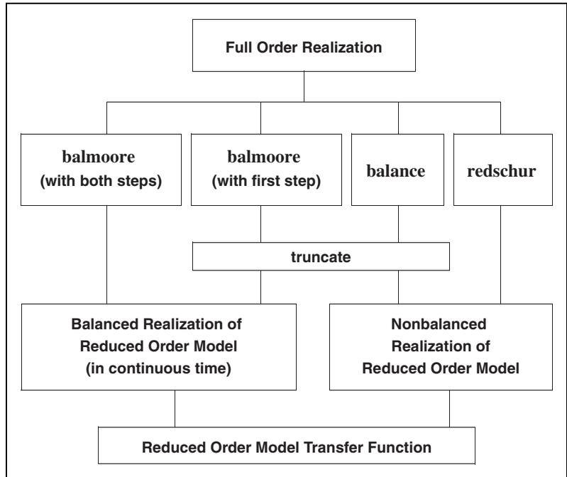
Figure 2-1. Different Approaches for Obtaining the Same Reduced Order Model
