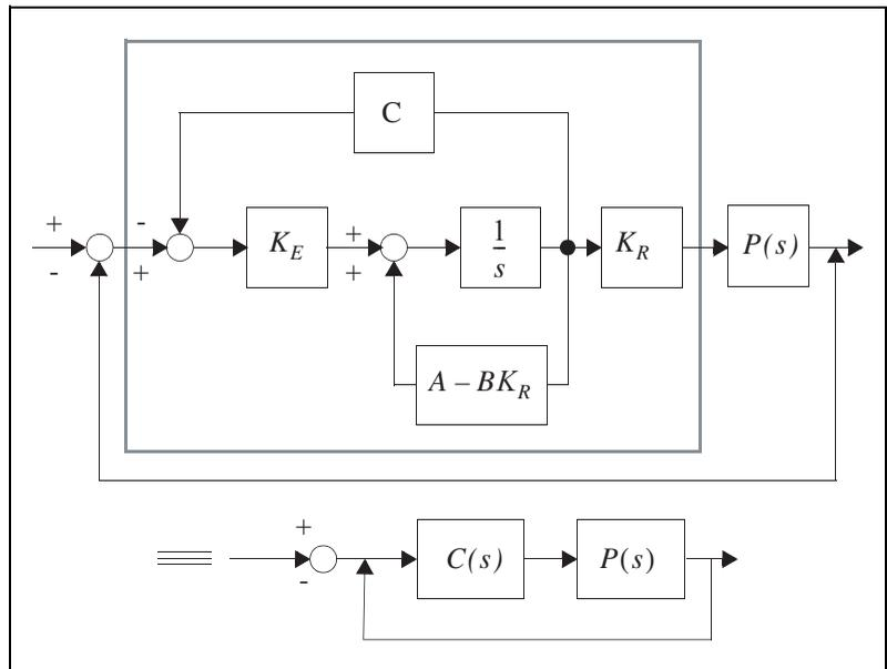
**Figure 4-2.**  $C(s)$  Implemented to Display Right MFD Representation
