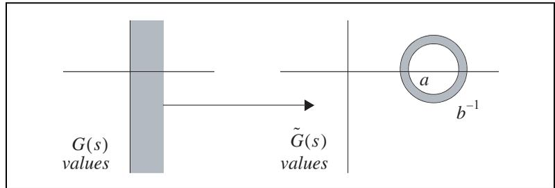
**Figure 3-2.** Bilinear Mapping from  $G(s)$  to  $\tilde{G}(s)$  (Case 1)
