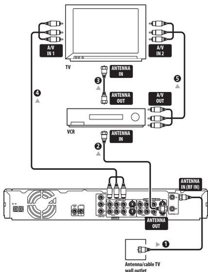
**1** Connect your TV antenna/cable TV outlet to the **ANTENNA IN (RF IN)** jack on this recorder.
