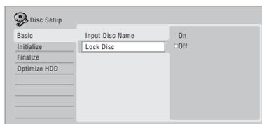
Set to **On** to prevent accidental recording, editing or erasing of the disc loaded. If you need to unlock the disc to make edits, select **Off**.
