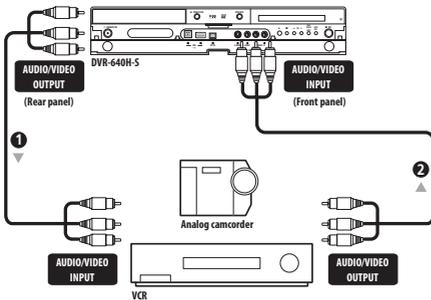
**1** Connect a set of audio and video inputs of your VCR or camcorder to a set of outputs on this recorder.
