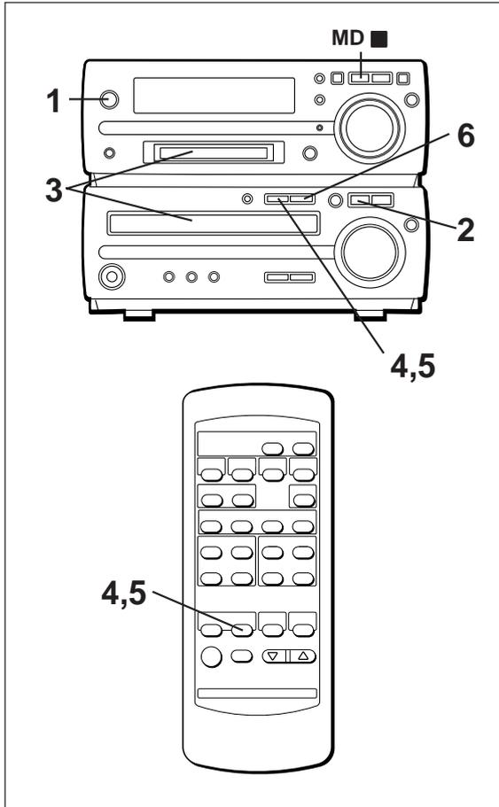
**1** Press the ON/STAND-BY button to turn the power on.
