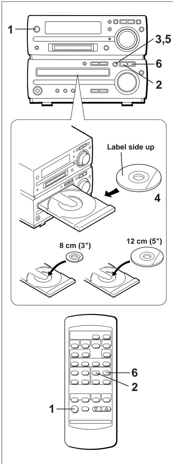
**1** Press the ON/STAND-BY button to turn the power on.
