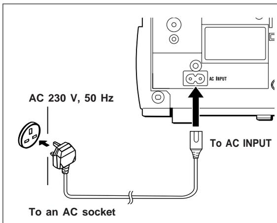
Connect the AC power lead to the AC INPUT socket, then connect its plug to an AC socket.
