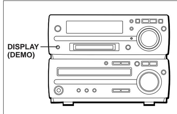
When the AC power lead is first connected, the unit will enter the demonstration mode and the words will scroll across the display continuously.
