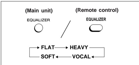
When the **EQUALIZER** button is pressed, the current mode setting will be displayed. To change to a different mode, press the **EQUALIZER** button repeatedly.
