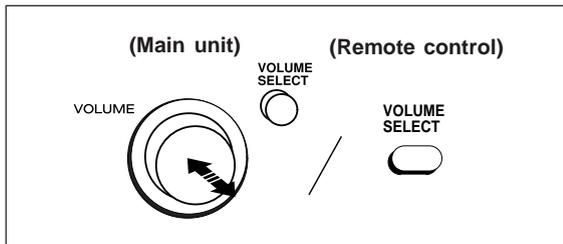
The **VOLUME** control automatically comes out when the power is turned on, and goes back when the unit is set to the stand-by mode.
