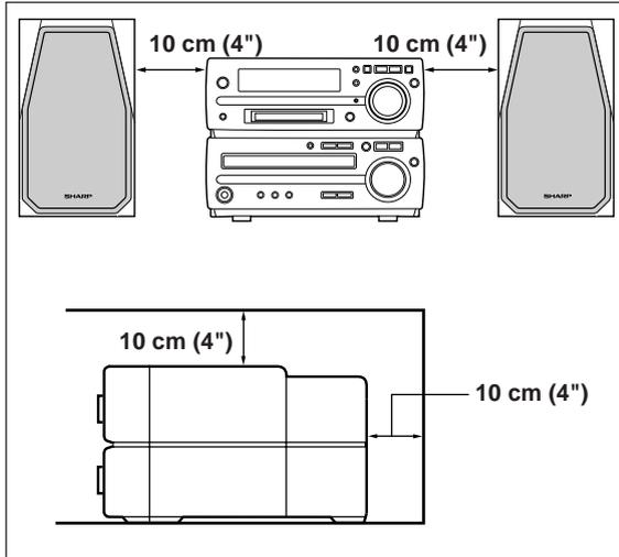
Be sure to keep space between the units for ventilation. Keep the top and the back of this unit at least 10 cm (4") away from the wall.
