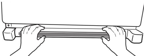
9. Using a 3/8" hex wrench, remove the leveling leg brackets from the bottom of the cabinet. Keep screws for later use.
