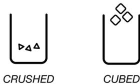
For crushed ice, cubes are crushed before being dispensed. This may cause a slight delay when dispensing crushed ice. Noise from the ice crusher is normal, and pieces of ice may vary in size. When changing from crushed to cubed, a few ounces of crushed ice will be dispensed along with the first cubes.
