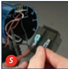
10. Replace hard plastic battery compartment cover. Make sure wires are not crushed.
