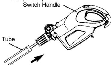
2. Push the tube into the motor housing until it snaps into place.
