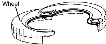
2. Attach the wheel to the trimmer. Make sure the wheel is fitted into the groove on the motor housing.
