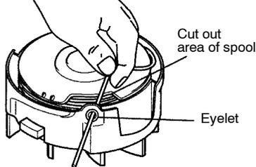
10. Remove line from notch and feed line through eyelet.
