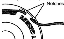
9. Place spool into hub with cut out area of spool in line with eyelet (see illustration).
