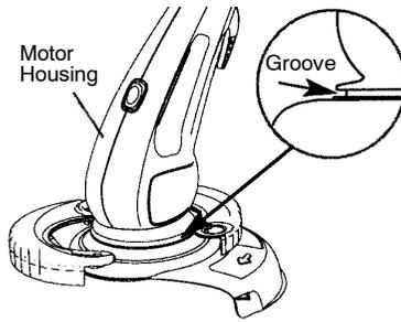
3. Clip the wheel together securely on the other side. The wheel should turn freely.
