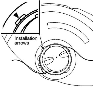
3. Twist the shield as illustrated until it snaps securely into place. Make sure the shield is assembled to the unit as shown in the illustration below and in the KNOW YOUR TRIMMER section of this manual.
