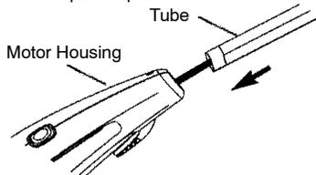
3. Try to remove tube from switch handle and motor housing. If the tube remains in place, it is properly snapped into place. If the tube will not remain in place, repeat steps 1 and 2. Push until the tube snaps into place.
