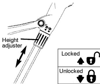
2. Adjust the length of the tube to the most comfortable operating position.
