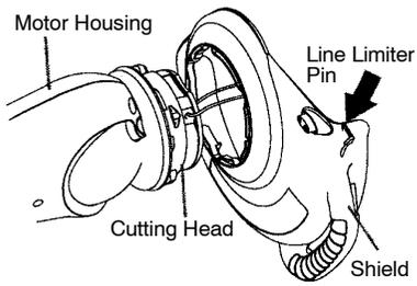
2. Align the installation arrow on the shield with the installation arrow on the motor housing as shown.
