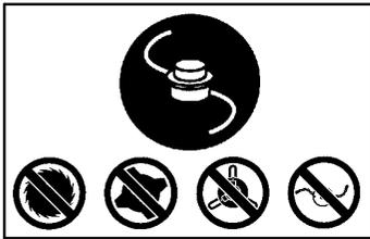
**⚠ DANGER:** Use only specified trimmer head, spool, and 0.065 inch (1.65 mm) recommended trimmer line. Never use blades, flailing devices, wire, rope, string, etc. Unit is designed for line trimmer use only. Failure to follow these instructions may result in serious injury.
