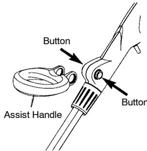
2. Push the assist handle over the buttons and release the buttons.
