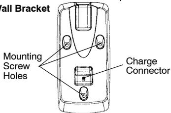
3. Ensure that when the trimmer is hung in the wall bracket, the bottom of the trimmer is within 4 inches (100 mm) of the ground. This will make it easier to hang the trimmer for charging and will also ensure that the wall bracket is within easy reach of an electrical outlet for plugging in the charger.
