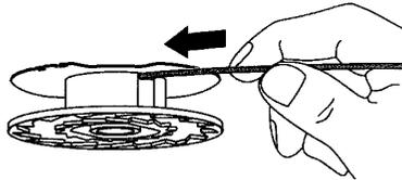
7. Wind the line evenly and tightly onto the spool. Wind in the direction of the arrow found on the spool.
