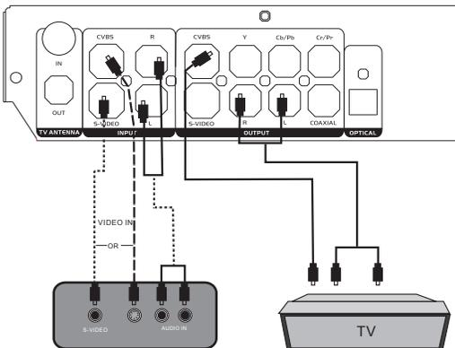
Connect your recorder with the S-Video cable, if the Signal source has an S-Video input. Do not connect the yellow video cable if using the S-Video cable.
