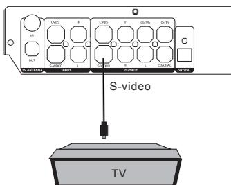
Connect your recorder with the S-Video cable, if the TV has an S-Video input. Do not connect the yellow video cable if using the S-Video cable.
