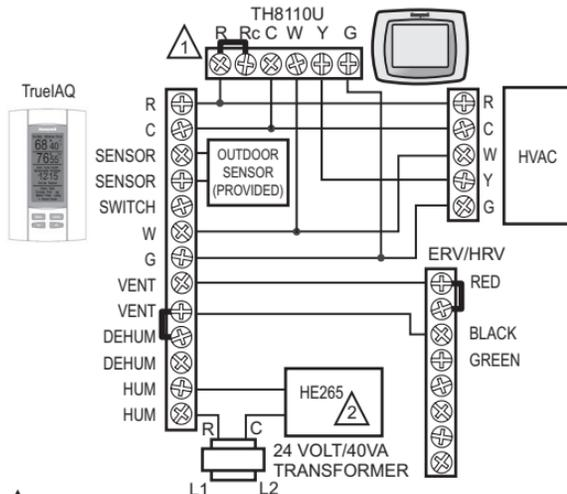
**1** IF A THERMOSTAT OTHER THAN A TH5110, TH5220, TH5320, TH6110, TH6220, TH6320, TH8110, TH8320 OR TH8321 IS USED, A RELAY MAY BE REQUIRED TO ISOLATE THE G WIRE.
