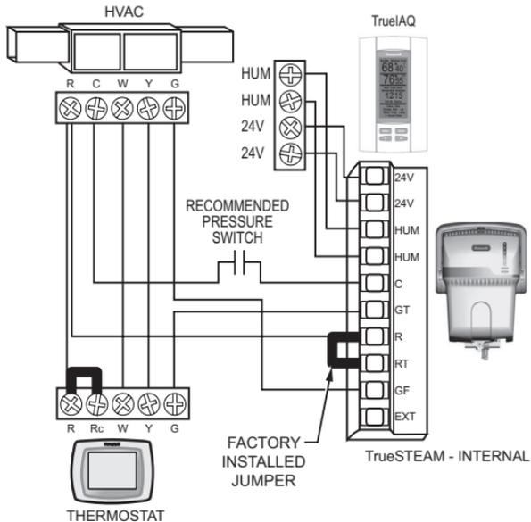
NOTE: IF PRESSURE SWITCH IS USED, ENSURE DIP 5 IS IN POSITION. M27341
