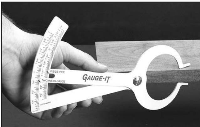
Figure 21. Model G2857 Thickness Gauge.
