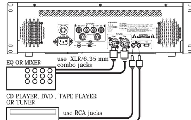
Connecting an equalizer or external signal processor
