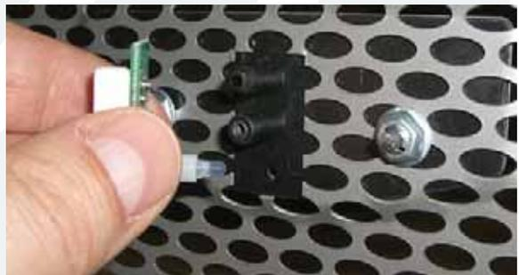
**6** Carefully remove the led PCB assembly from the back side of the grill.
