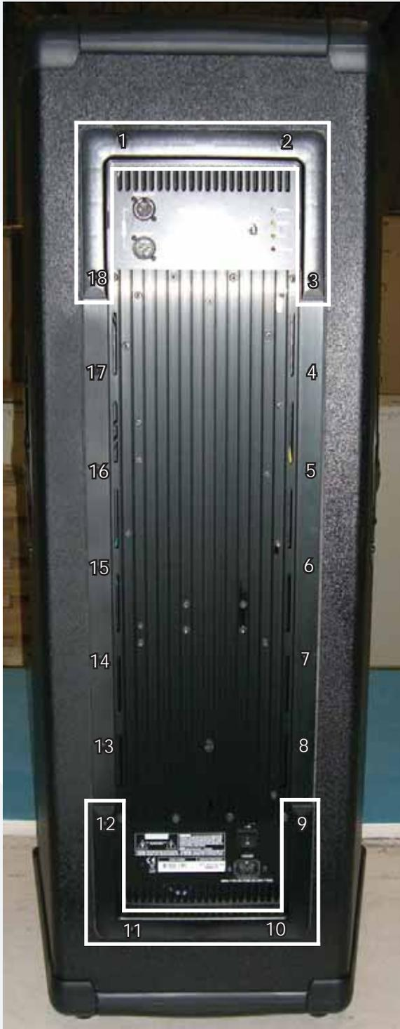
**1** Eighteen screws need to be removed from the amplifier assembly using the phillips head screwdriver. The amplifier assembly is capped by two cover plates outlined above.
