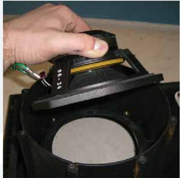
**7** The mid frequency driver easily lifts right off of the horn. Replace with the new driver (part #0013897) and follow the same steps as above, but backwards 7 to 1. Power up the SA1530z and the new driver should now be pumping out those mids again. Right on, you just replaced a mid frequency driver!
