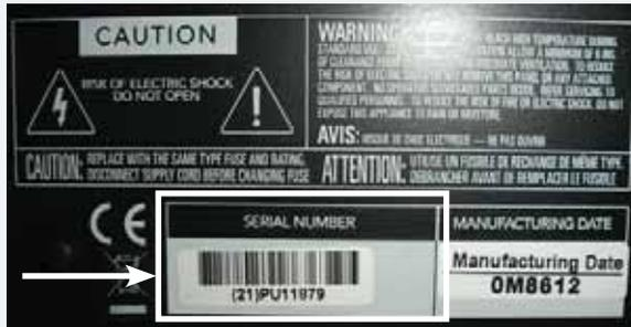
**8** Place the new amplifier assembly (part #0013839-00) where the old one was. Follow the same steps as above, but backwards 7 to 1. Remove the serial number from the faulty amplifier assembly (as shown in picture above) and place on the new amplifier assembly. Power up the SA1530z and relish in the fact that you just replaced an amplifier assembly. Hats off to you for a job well done!
