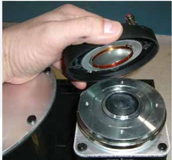
**5** The diaphragm and plate adapter are easily removed from the horn assembly. They may not be broken down any further. Place the new diaphragm (part # coming soon) and plate assembly where the old one was. Follow the same steps as above, but backwards 4 to 1. Power up the SA1530z and the new diaphragm should now be pumping out those highs again. Sweet, you just replaced a diaphragm!
