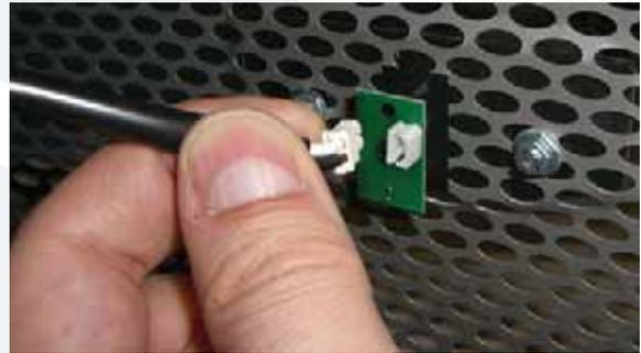
**4** Carefully remove the cable attached to the led PCB assembly.
