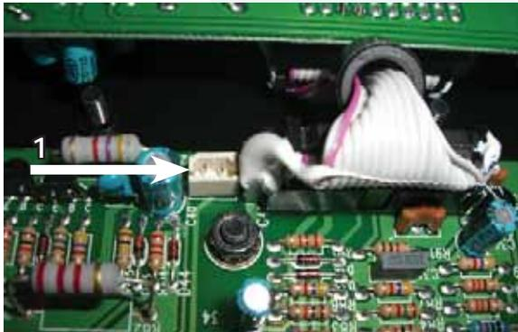
**6** Closeups of the led PCB cable and connector are shown above. The black wire of the cable is closest to the ribbon cable. The cable only fits in one way.
