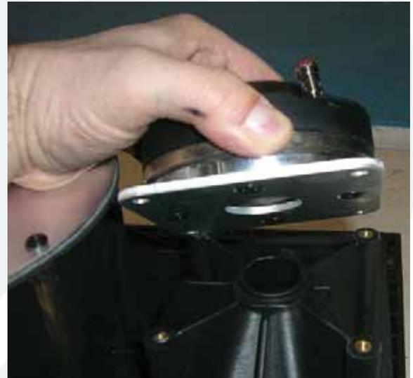
10 The high frequency driver should easily lift right off of the horn assembly. Holding down the horn assembly with one hand while lifting up on the driver with the other hand may help.
