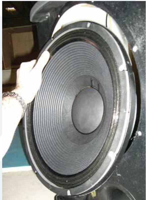
**2** Eight screws and washers need to be removed from the woofer using the 4mm allen wrench.
