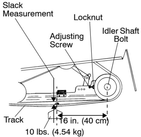
9. Start the engine and slowly rotate the track at least five revolutions. Let the track come to a stop (do not apply brakes).
