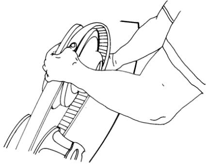
2. Turn the driven clutch moveable sheave clockwise while pushing inward and forcing the belt down between the sheaves.
