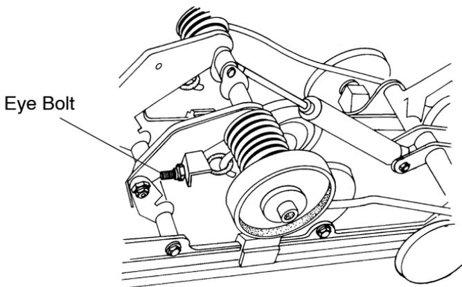
**NOTE:** Rear spring settings will affect ski-to-ground pressure. If ski pressure is too light it may be desirable to tighten the rear springs for an increase in ski-to-ground pressure.
