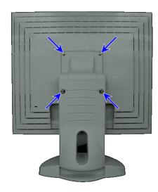
3. Remove the four mounting plate retaining screws. One screw at each corner. Lift the base up and away from the monitor.
