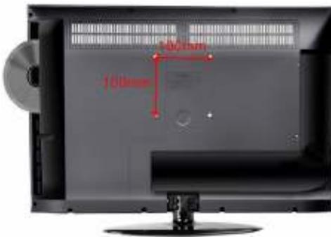
Mounting Specification : **100mm x 100mm** using screw size **M4**. Length of screw should not exceed **8mm**. Please Note : The **8mm** length of screw refers to how deep the screw can go inside the mounting holes. When you're buying screws, you should add the original 8mm to the thickness of your mounting plate in order to get the total screw length.
