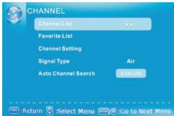
3. Use the ▲ or ▼ buttons to highlight the signal type and press ◀ or ▶ to select your connection either AIR or CABLE.
