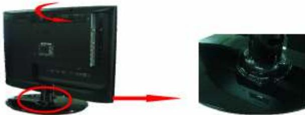
2. Rotate the HDTV (counter-clockwise) as the picture has shown until you hear a clicking sound from the base. Afterwards, the HDTV will be ready for use.
