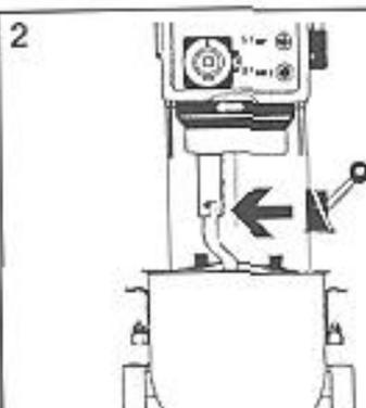
2 Place the mixing tool in the bayonet shaft. The pin of the tool must be turned into the bayonet hole.
