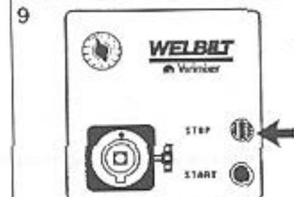
9 Stop the mixer by pressing the red stop button <STOP>
