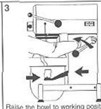
3 Raise the bowl to working position by pulling the handle forward. Ensure that the bowl is placed correctly while the bowl is lifted.
