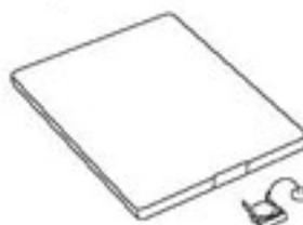
Insert battery holder into controller.
