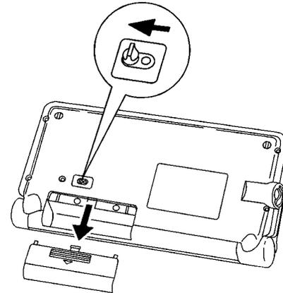
4. Remove the old batteries by pulling the ribbon tab.
