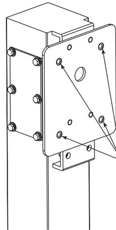
Mount the LTC 9540/xx Wall Bracket Using These Holes
