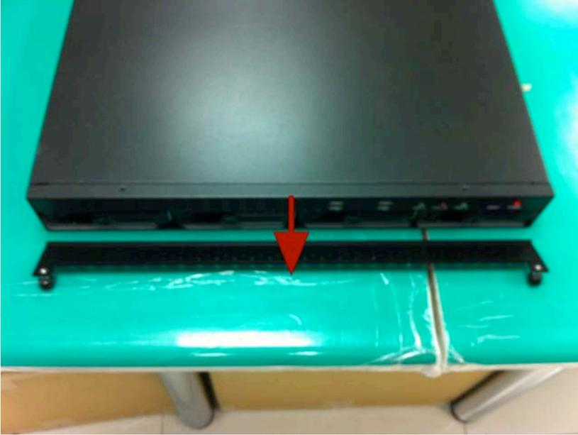
Simply pull to remove the front plate once the screws are loosened from the unit.
