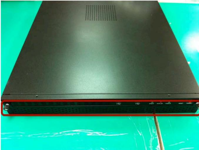
Start by removing the front plate.
