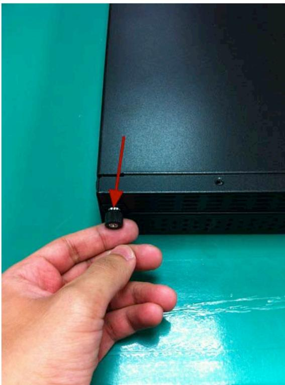
To remove the front plate, turn the tool-less screws on both sides counter-clock wise to loosen it from the unit. Please note the screws will still be attached to the front plate even after the screws are completely loosened from the unit.
