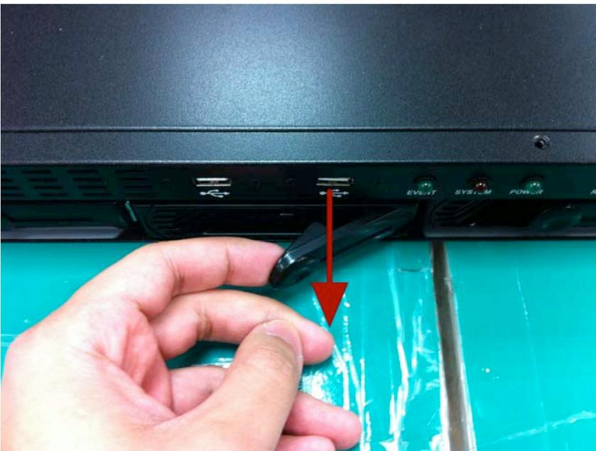
Release the HDD tray by pulling the latch.
