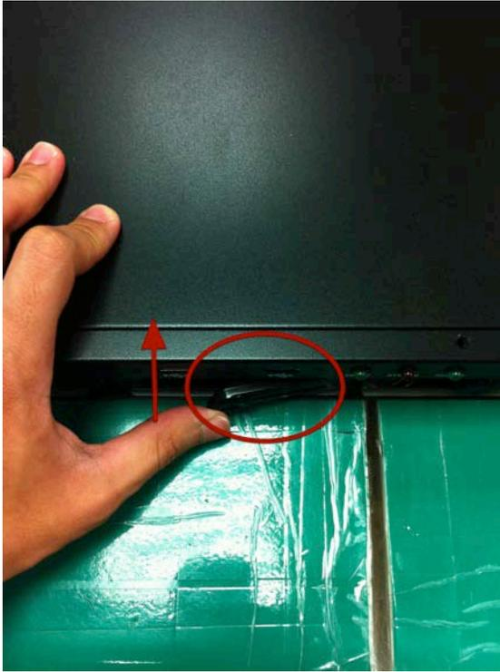
Secure the HDD tray by pushing in the latch, which locks the HDD tray with the unit.
