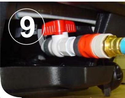
Close the discharge valve handle and disconnect the drain hose from the discharge valve.
