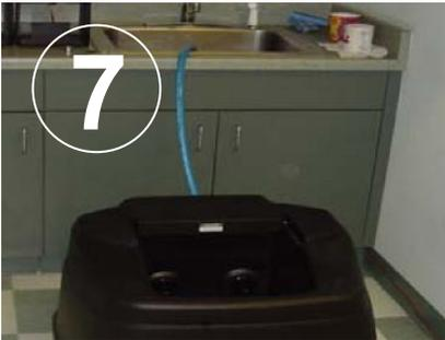
Run the pump until the water stops draining out of the hose. It is normal for a low volume of water to run out of the jets while the Spa is draining.
