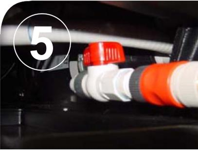
Open the discharge valve by turning the handle so that it is straight with the discharge valve.
