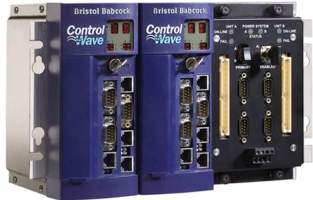
Data Backup – The standby CPU is automatically updated via Ethernet link to the on-line unit. In addition to real-time data backup, ControlWave also provides backup of all alarm events and the distributed historical database. These functions are all pre-configured, and no control programming is required to implement the redundancy functionality.
