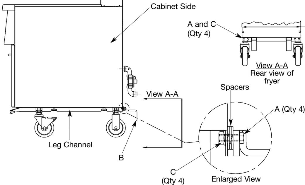
**CAUTION:** During assembly of Item B, sides of cabinet should be parallel. Clearance in mounting holes on cabinet sides, leg channels and bumper guard will allow adjustment when attaching hardware. Tighten bolts and nuts at the end of installation.
