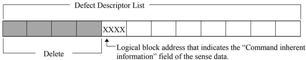
2. Change the “Defect List Length” in the header and add the new ”Defect descriptor list” corrected in 1), then reissue the REASSIGN BLOCKS command.
