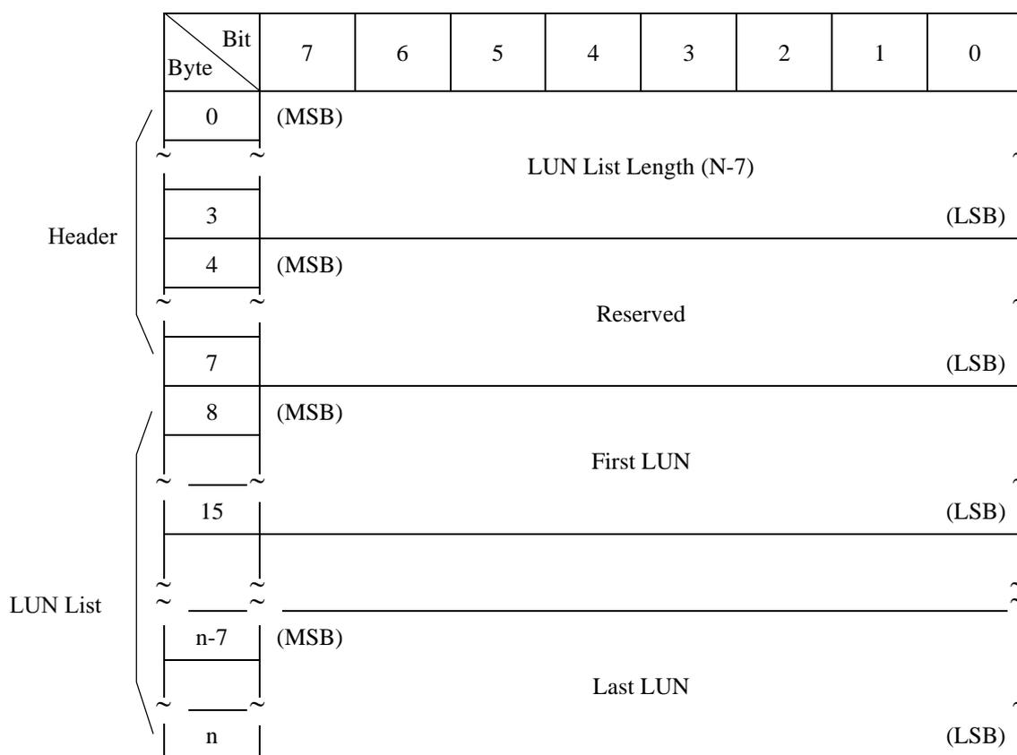
The "LUN List Length" field shall contain the length in bytes of the LUN list that is available to be transferred. The "LUN list length" is the number of logical unit numbers in the logical unit inventory multiplied by eight. If the allocation length in the command descriptor block is too small to transfer information about the entire logical unit inventory, the LUN list length value shall not be adjusted to reflect the truncation.
