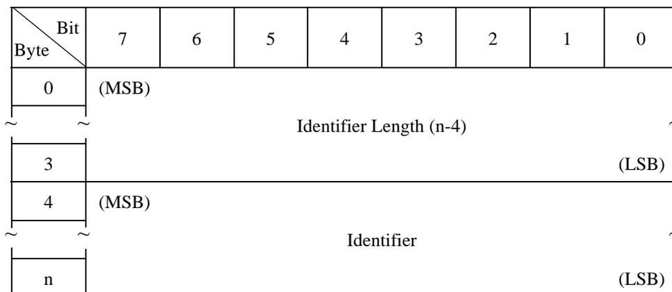
The "Identifier Length" field specifies the length in bytes of the "Identifier" field.
