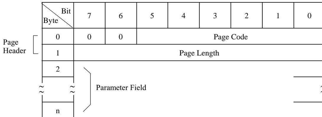
**Figure 3.9 MODE SELECT EXTENDED command (Group 2) parameter configuration**
