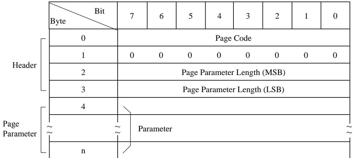
**Figure 3.18 SEND DIAGNOSTIC command: parameter list configuration**
