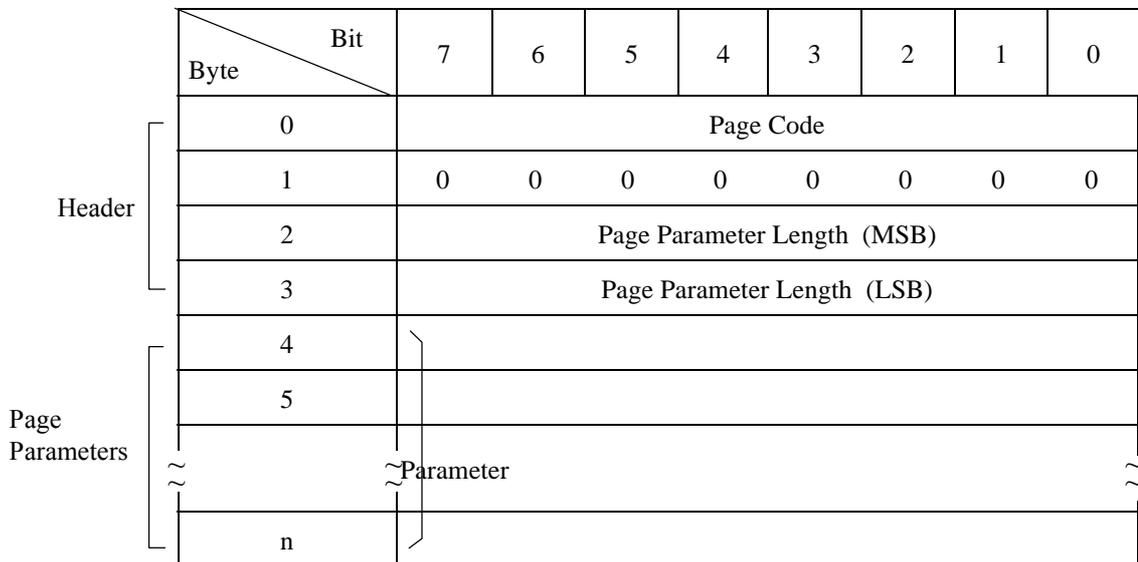
**Figure 3.21 RECEIVE DIAGNOSTIC RESULTS command: Response data configuration**
