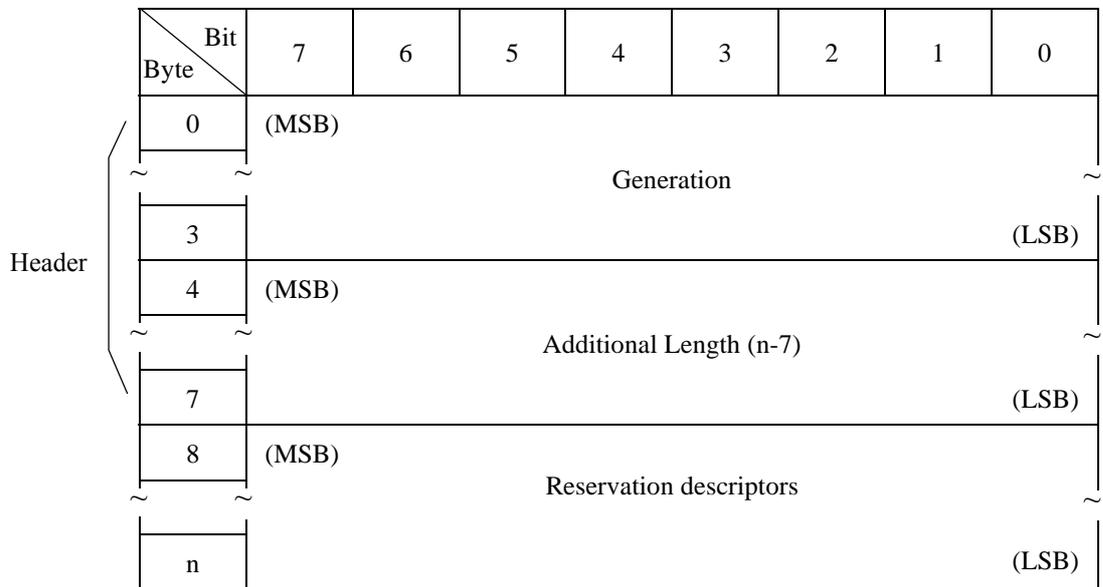
The "Generation" field contains the same value defined in the parameter data field of the READ KEYS service action of the PERSISTENT RESERVE IN command (See Section 3.1.18.2).
