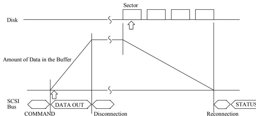
**Figure 2.3 Example of data buffer operation during write**
