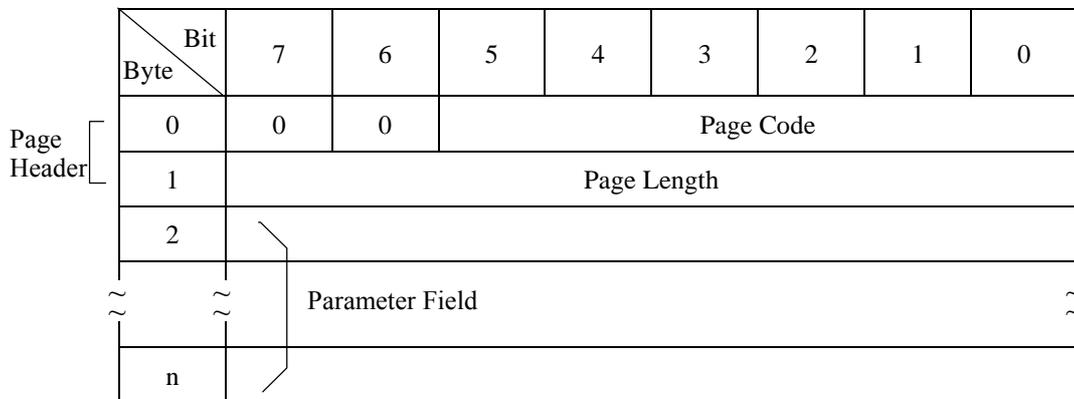
**Figure 3.8 MODE SELECT command (Group 0) parameter configuration**
