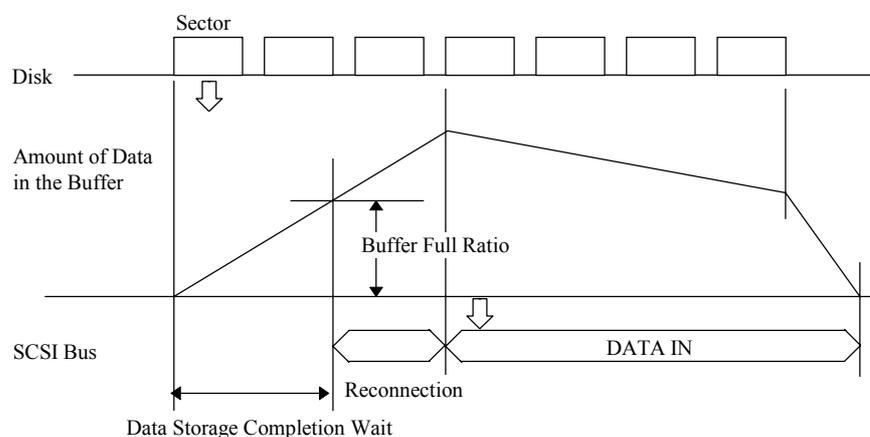
**Figure 2.2 Example of data buffer operation during read**
