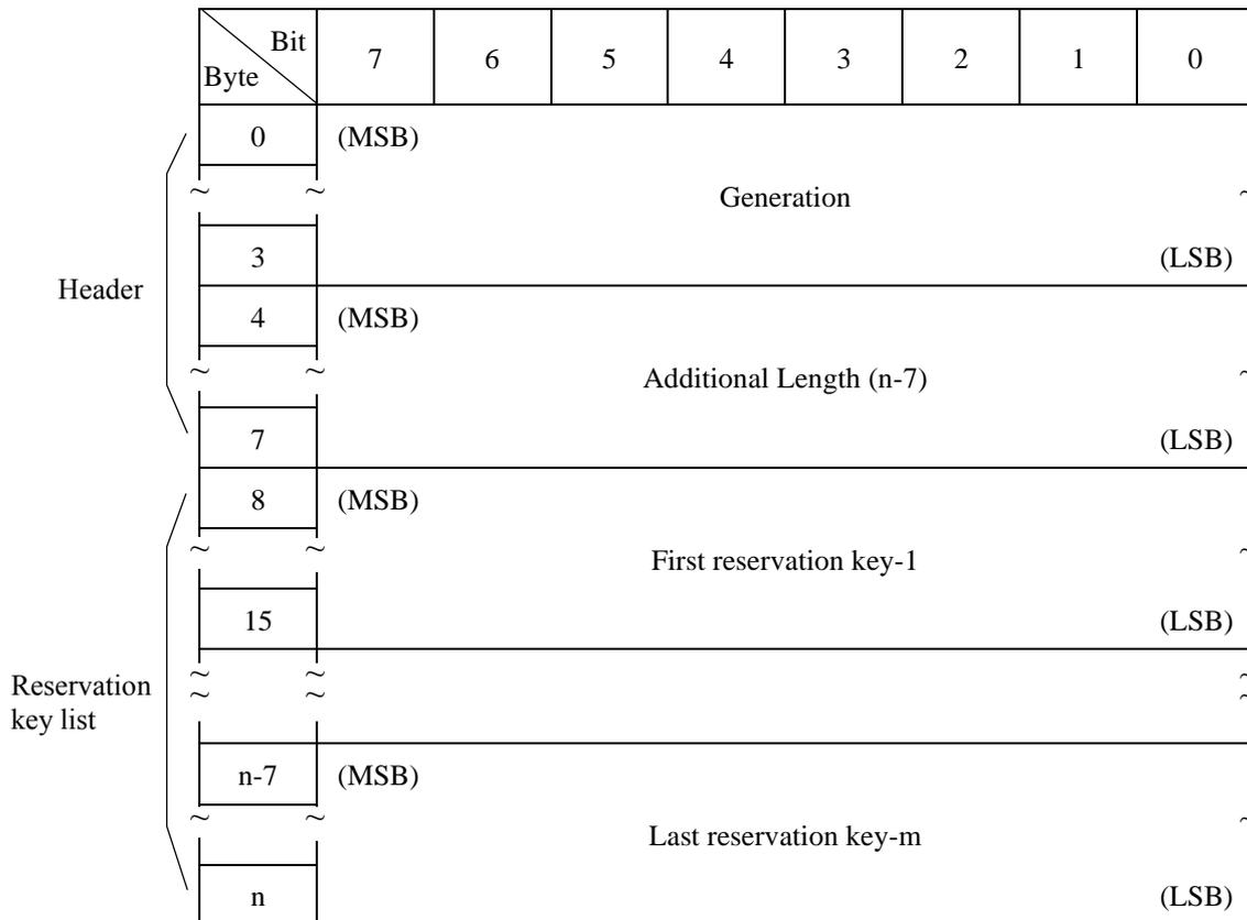
The "Generation" field contains a 32-bit counter value maintained by the driver. This counter value is incremented every time the PERSISTENT RESERVE OUT command requests execution of the REGISTER, REGISTER AND IGNORE EXISTING KEY, CLEAR, PREEMPT, or PREEMPT AND ABORT service action.
