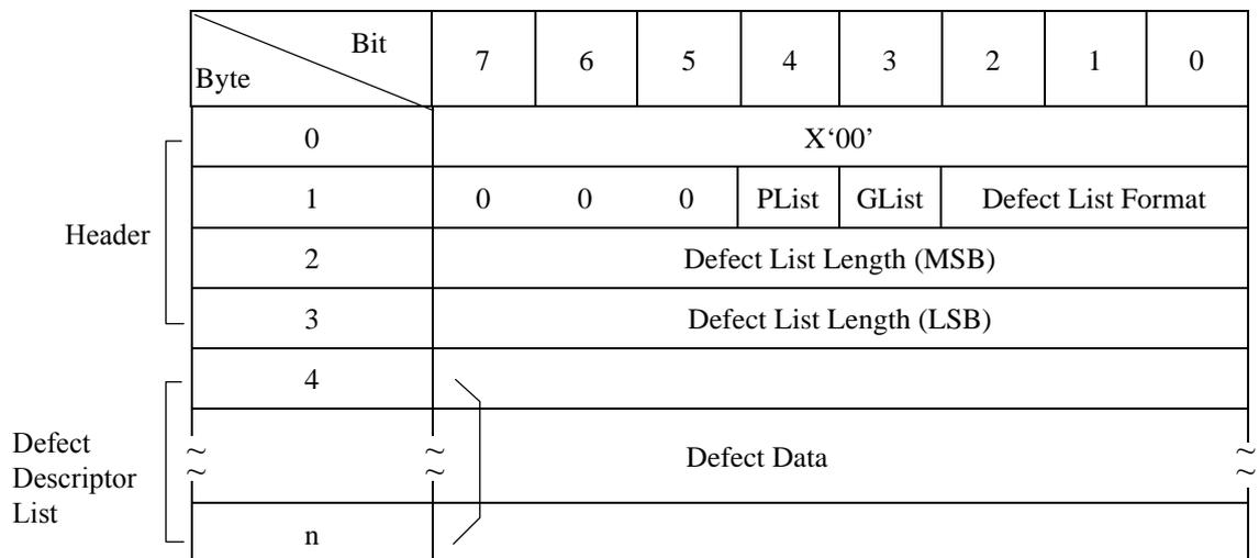
**Figure 3.17 READ DEFECT DATA command: Defect data configuration**
