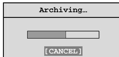
When the unit is finished archiving this message box will appear. Press the **Enter** button to acknowledge the message and complete the archiving process.
