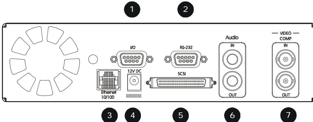
1. **I/O Port:** For connecting peripheral devices such as alarm devices, alarm relays, or the VEXT connection.
