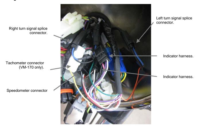
Some stock wiring harnesses have the wires going to one of the turn signals reversed and the supplied cross over harness must be used to fix the connection. If the left turn signal indicator does not work, insert the cross over harness in line on that side.
