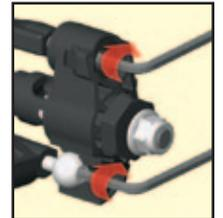
**Rear Toe Adjustment:** Rear toe-in is adjusted in the same way as front toe-in, by adjusting the depth of the pivot balls in the arms. Increasing rear toe-in will add stability to the model and make the model handle less aggressively (to use racing terminology, the model will have "less steering"). Reducing toe-in will "loosen" the rear of the model, making it more likely to spin-out (oversteer). Rear toe-out is not recommended, as it will cause erratic handling.
