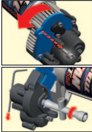
The slipper clutch is adjusted using the spring-loaded locknut on the slipper shaft. Use the supplied universal wrench. To tighten or loosen the slipper nut, insert the 1.5mm hex wrench into the hole in the end of the slipper shaft. This locks the shaft for adjustments. Turn the adjustment nut clockwise to tighten (less slippage) and counter-clockwise to loosen (more slippage).
