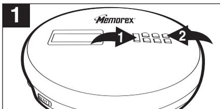
With a CD inserted, press the PLAY/PAUSE (▶||)/POWER ON button ❶ to turn the unit on. Press the MODE button ❷ twice; the Repeat All indicator
