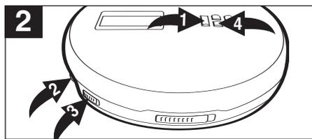
Press the PLAY/PAUSE (▶||)/POWER ON button ❶ to begin playback. The unit will play all the tracks in random order. Adjust the VOLUME control ❷ and DBBS switch ❸ as desired. When all the tracks have been played, the unit will stop. Press the STOP (■)/POWER OFF button ❹ to stop Random playback.
