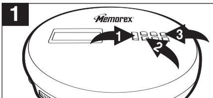
With a CD inserted, press the PLAY/PAUSE (▶||)/POWER ON button ❶ to turn the unit on and press the STOP (■)/POWER OFF button ❷ to stop auto playback. Press the MODE button ❸ four times; the RAND indicator will appear in the display.
