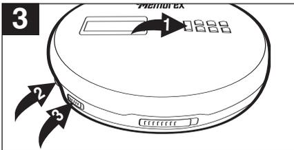
Press the PLAY/PAUSE (▶||)/POWER ON button ❶ to begin Programmed playback and adjust the VOLUME control ❷ and DBBS switch ❸ as desired.
