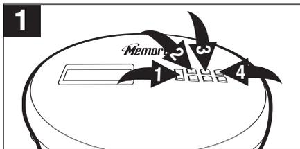
With a CD inserted, press the PLAY/PAUSE (▶||)/POWER ON button ❶ to turn the unit on, then select a track using the SKIP/SEARCH ◀◀ ❷ or ▶▶ ❸ button. Press the MODE button ❹ once; the Repeat 1 indicator
