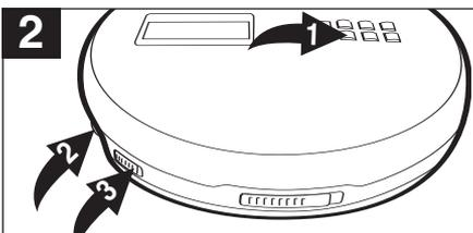
The unit will then play all the tracks on the CD over and over until the STOP (■)/POWER OFF button ❶ is pressed. Adjust the VOLUME control ❷ and DBBS switch ❸ as desired.
