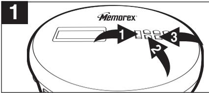
With a CD inserted, press the PLAY/PAUSE (▶||)/POWER ON button ❶ to turn the unit on and press the STOP (■)/POWER OFF button ❷ to stop auto playback. Press the PROG button ❸; the PROG indicator will blink in the CD display.
