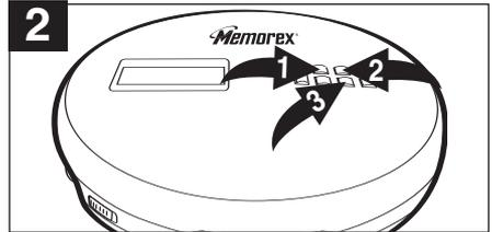
Select the first track to be played back using the SKIP/SEARCH ◀◀ ❶ or ▶▶ ❷ button, then press the PROG button ❸ again. Repeat this step to program additional tracks up to a maximum of 24 tracks.
