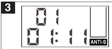
The Anti-Shock System will start automatically, the sound will mute for a moment and the display will show the Anti-Shock indicator with no bars in it.
