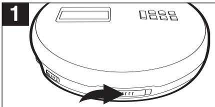
Open the CD compartment lid by sliding the CD OPEN switch to the right. Gently press a disc, label side up, onto the spindle until it locks in place. Close the CD compartment lid. Insert headphones into the PHONES jack.
