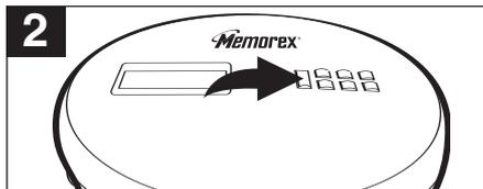
While the unit is off, press the PLAY/PAUSE (▶||)/POWER ON button to start playback. To pause **PLAYBACK**, press the PLAY/PAUSE (▶||)/POWER ON button again, the display will blink. Press once again to resume playback.
