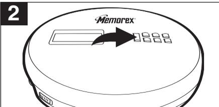
With a CD inserted, press the PLAY/PAUSE (▶||)/POWER ON button to turn the unit on.
