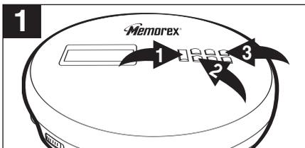
With a CD inserted, press the PLAY/PAUSE (▶||)/POWER ON button ❶ to turn the unit on and press the STOP (■)/POWER OFF button ❷ to stop auto playback. Press the MODE button ❸ three times; the INTRO indicator will appear in the display.
