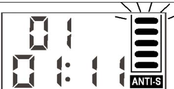
If no more vibration occurs, the music signals are once again stored into the memory and the indicator returns to full. When the memory is full, the top bar will blink and the disc rotation speed will drop to save power consumption.
