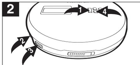
Press the PLAY/PAUSE (▶||)/POWER ON button ❶ to begin playback. The unit will play the first 10 seconds of each track. Adjust the VOLUME control ❷ and DBBS switch ❸ as desired. Press the STOP (■)/POWER OFF button ❹ to stop Intro playback.
