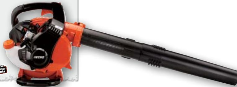
**"Rotational Control"** design reduces the effort required to keep the blower from rotating in towards the operator's legs (like most handheld models do) and actually delivers a slight pull away from the operator (green section). The effect makes the blower easier to handle and reduces stress on the operator's arm.
